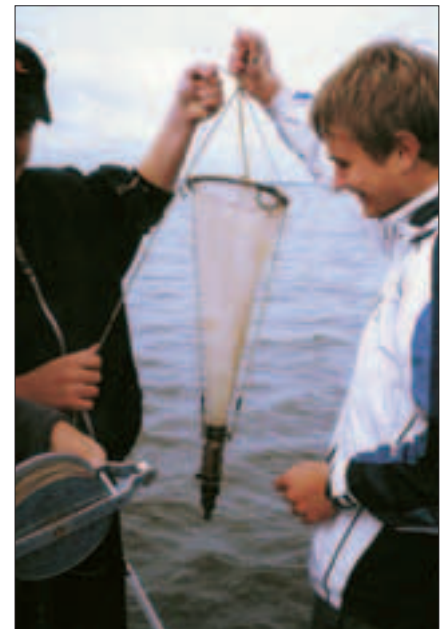
The water sampler takes samples from the different water layers up to 40 metres.
