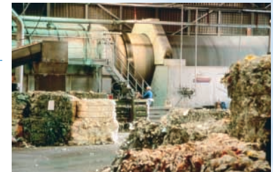
Paperfibres are separated in drum pulpers
