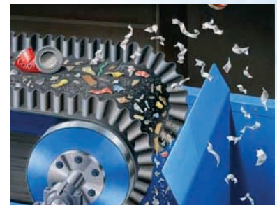
Mode of action of an eddy-current separator (Illustration with friendly permission from Master Magnets Ltd.)
