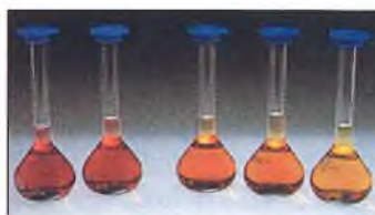
14.3) Visual comparison of the colours for the determination of phosphates
